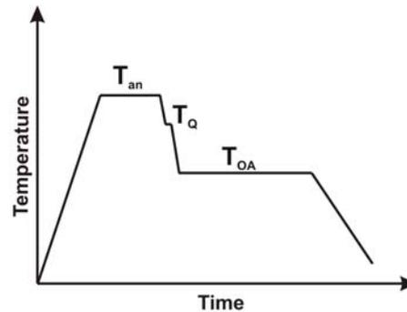
*Figure 2. Schematic representation of applied annealing cycles*
