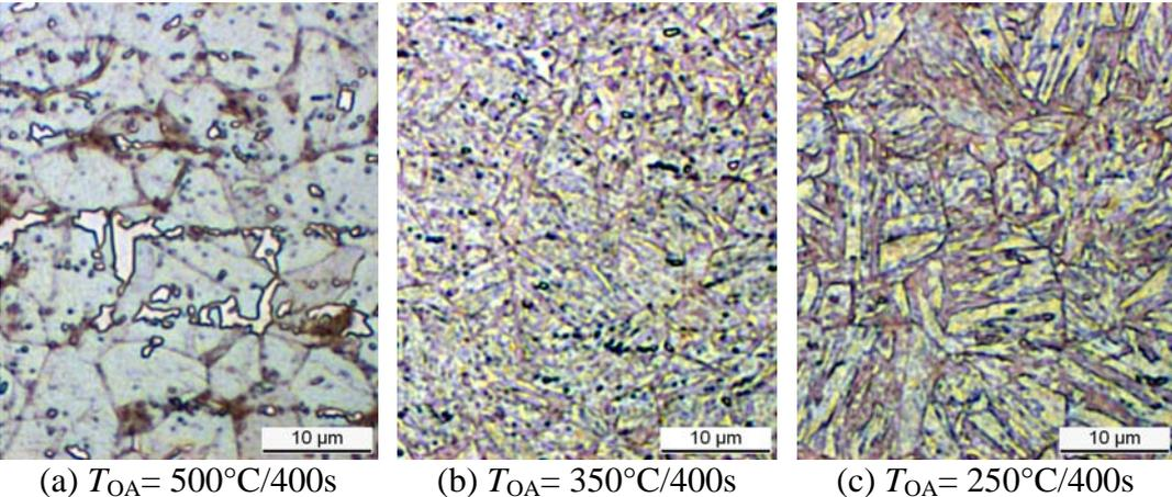
**Figure 7.** Influence of overaging temperature on the microstructure of steel B ( $T_{an} = 840^{\circ}\text{C}/120\text{s}$ ,  $T_Q = 750^{\circ}\text{C}$ )
