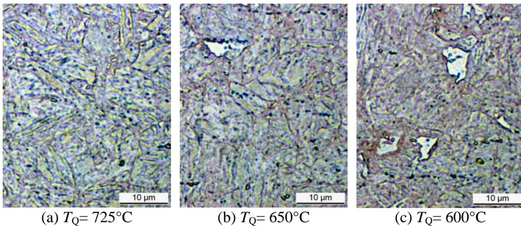
**Figure 4.** Influence of quenching temperature on the microstructure of steel B ( $T_{an} = 840^{\circ}\text{C}/120\text{s}$ ,  $T_{OA} = 300^{\circ}\text{C}/400\text{s}$ )
