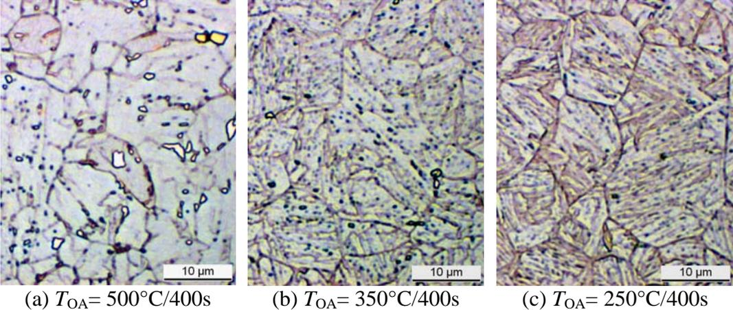
**Figure 6.** Influence of overaging temperature on the microstructure of steel A ( $T_{an} = 840^{\circ}\text{C}/120\text{s}$ ,  $T_Q = 750^{\circ}\text{C}$ )
