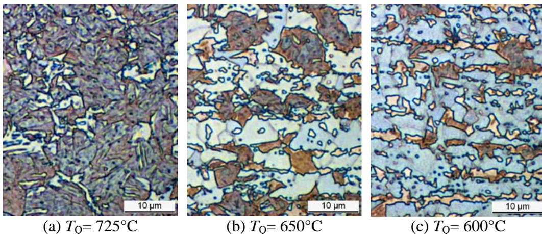
**Figure 5.** Influence of quenching temperature on the microstructure of steel C ( $T_{an} = 840^{\circ}\text{C}/120\text{s}$ ,  $T_{OA} = 300^{\circ}\text{C}/400\text{s}$ )
