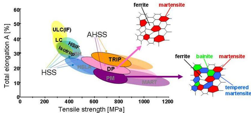
**Figure 1.** Ductility–strength relationship of mild and high strength steels with schematic illustration of dual-phase and partial-martensitic microstructure
