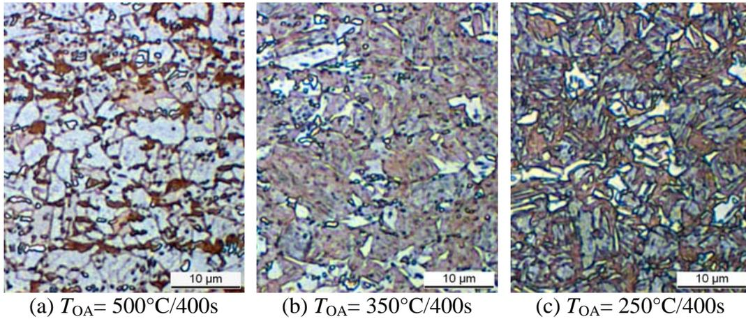
**Figure 8.** Influence of overaging temperature on the microstructure of steel C ( $T_{an} = 840^{\circ}\text{C}/120\text{s}$ ,  $T_Q = 750^{\circ}\text{C}$ )
