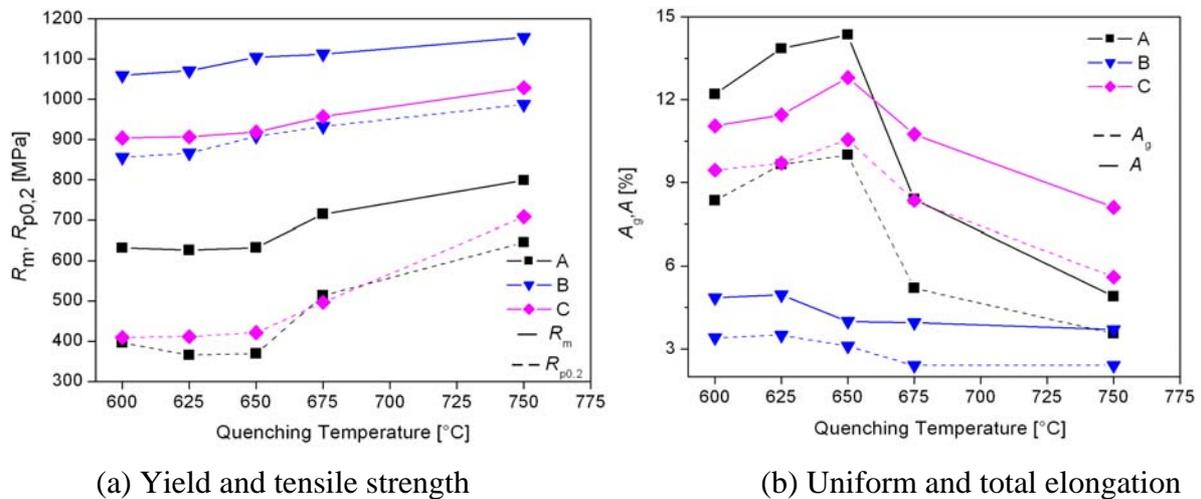
**Figure 9.** Influence of the quenching temperature on the mechanical properties ( $T_{an} = 840^{\circ}\text{C}/120\text{s}$ ,  $T_{OA} = 300^{\circ}\text{C}/400\text{s}$ )
