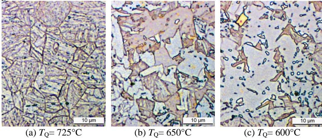
**Figure 3.** Influence of quenching temperature on the microstructure of steel A ( $T_{an} = 840^{\circ}\text{C}/120\text{s}$ ,  $T_{OA} = 300^{\circ}\text{C}/400\text{s}$ )
