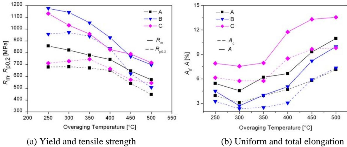
**Figure 10.** Influence of the overaging temperature on the mechanical properties ( $T_{an} = 840^{\circ}\text{C}/120\text{s}$ ,  $T_Q = 750^{\circ}\text{C}$ )
