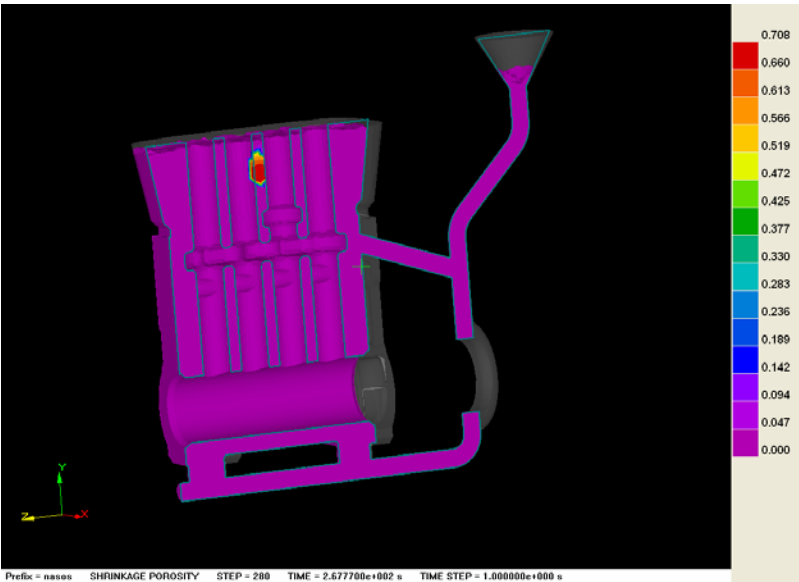
Fig. 5. Probability of formation of shrinkable defects (porosity) in casting alloy AK9 with simulation data of ProCAST
