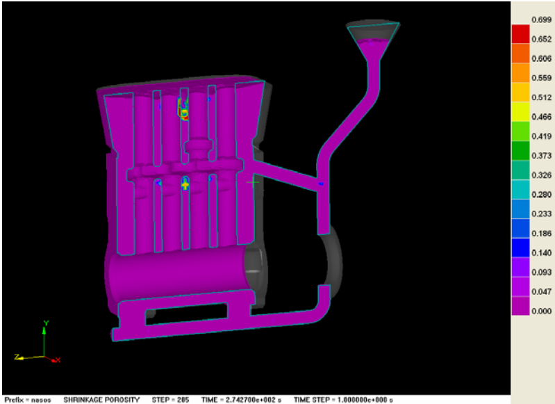
Fig. 6. Probability of formation of shrinkable defects (porosity) in casting with use of experimental data about phase transitions of alloy AK9
