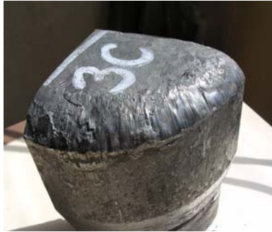
Picture n°.2 The extruding punch head, close-up of the face, R20 radius and side surface of the punch head
