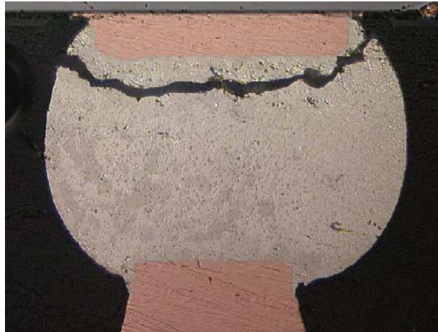
**Fig. 3** Optical micrograph of a failed Sn-3.5Ag solder joint after experiencing thermomechanical fatigue [5]
