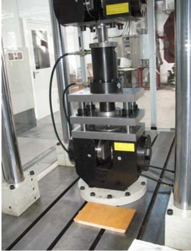
**Figure 2** Instrumented HE device implemented in the tensile testing machine type W+B 600
