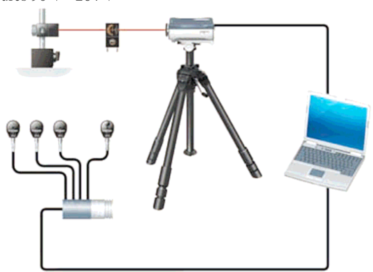
Fig. 6 Workplace of Renishaw XL 80 with integrated PC and compensator unit XC 80
