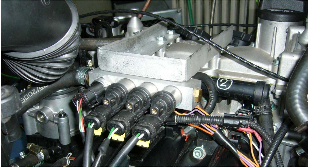
Figure 2 Detail of CNG common rail with CNG injectors, which was displaced close to cylinder head and original fuel rail for gasoline.
