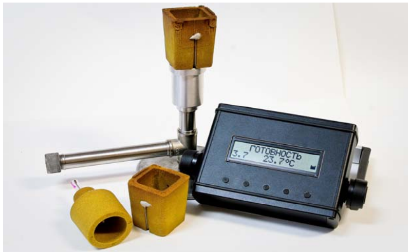
Fig. 2 Appearance of microprocessor system for the thermal (CA-CCA) analysis of cast alloys
