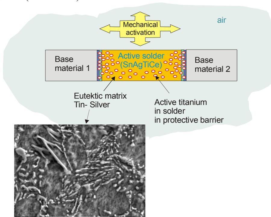
**Fig. 6.** Scheme of fluxless mechanical activation in the air (S-Bond process [6])
