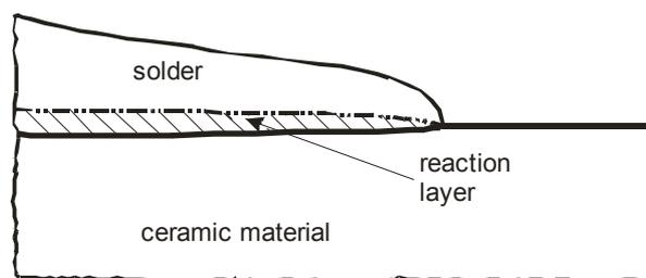
**Fig. 1.** *Scheme of formation of reaction layer on ceramic material*
