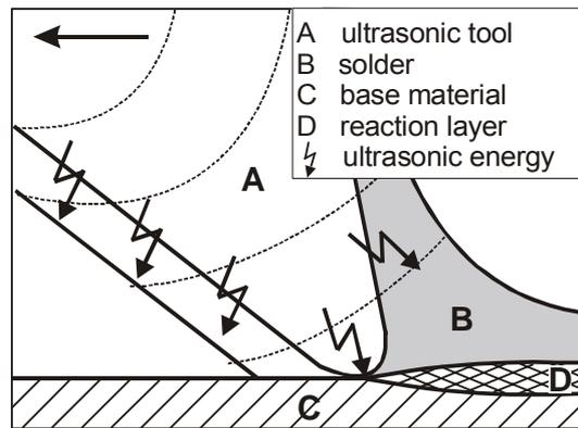
**Fig. 9.** Schematic representation of activation of surface of soldered material with US tool [7]
