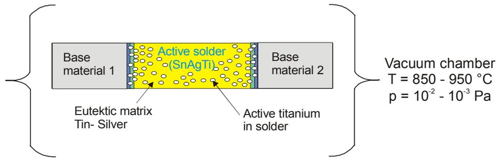
**Fig. 3.** Scheme of soldering with high-temperature activation in vacuum [4]
