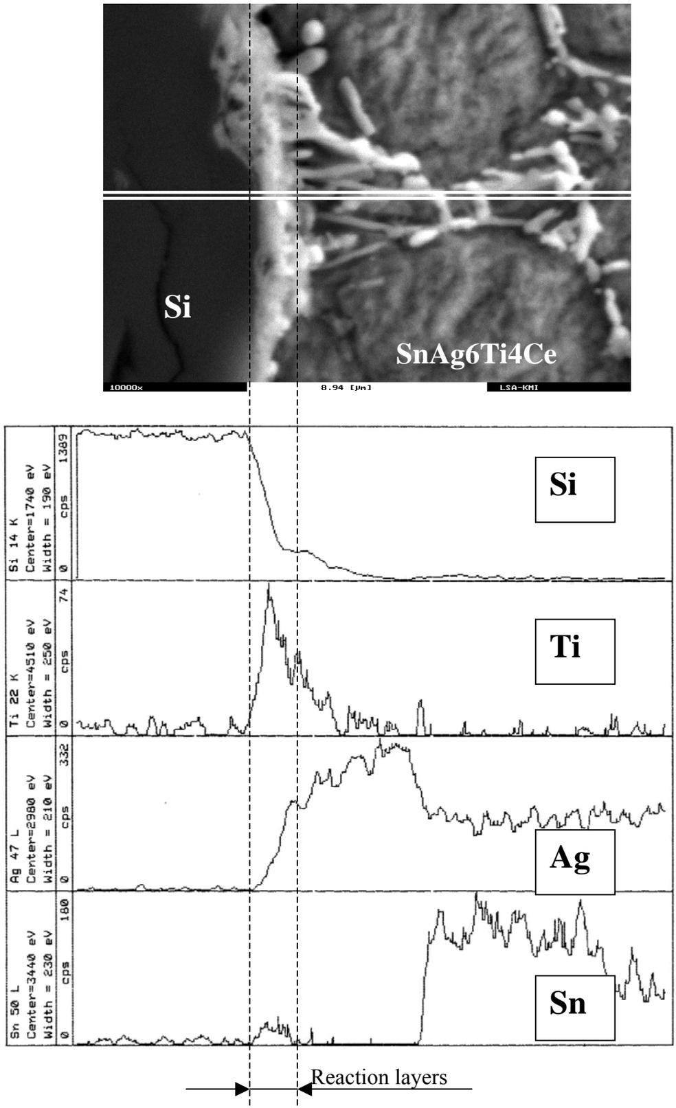
**Fig. 11.** Microstructure Si – SnAg<sub>6</sub>Ti<sub>4</sub>Ce solder joint and the concentration profiles of elements in this boundary [8]
