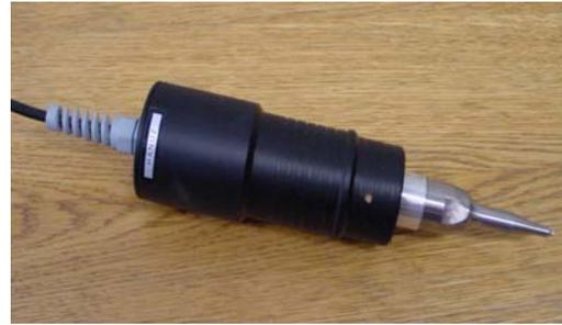
**Fig. 8.** Ultrasonic generator and ultrasonic head of experimental equipment for ultrasonic activation
