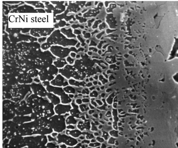
**Fig. 5.** Diffusion zone and solubility zone of CrNi steel in Sn solder
