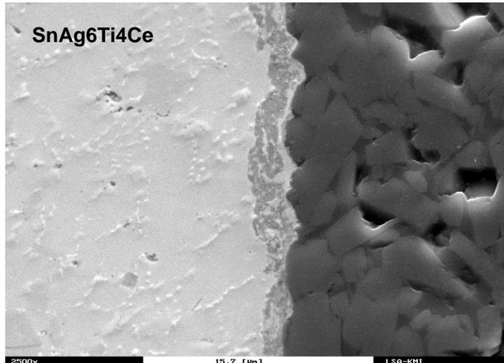
**Fig. 10.** Microstructure of  $Al_2O_3$  joint with SnAg6Ti4Ce solder in polished condition
