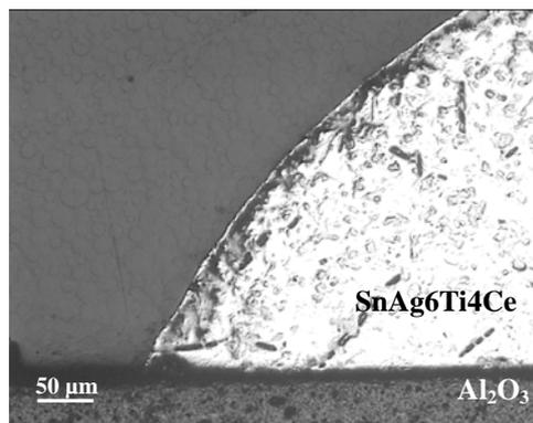
**Fig. 2.** A droplet of SnAg6Ti4Ce solder on  $Al_2O_3$  substrate with wetting angle of 62°
