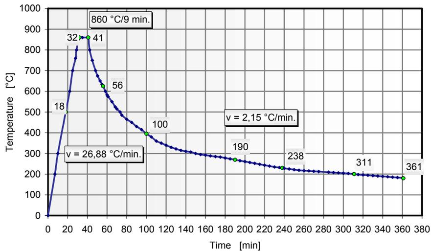
**Fig. 4.** Working cycle of soldering in vacuum furnace type of PZ 810
