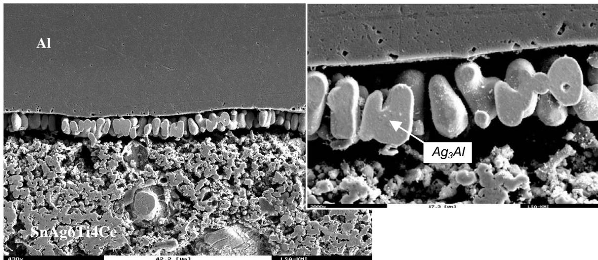
**Fig. 7.** Microstructure of joint of high purity Al with SnAg6Ti4Ce solder after deep etching of matrix
