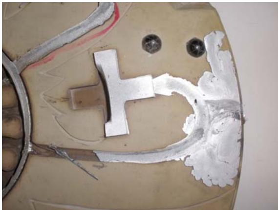
Fig. 10. Close up of mould with fin in parting plane
