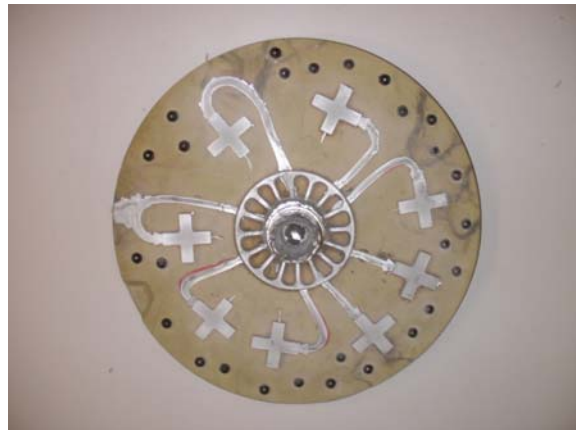
Fig. 11. Mould with all cavities filled
