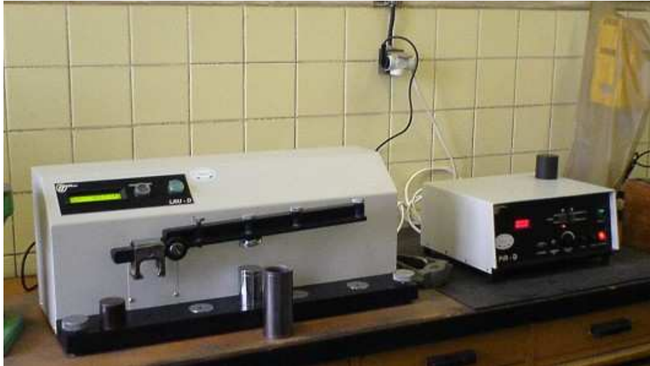
Fig. 1. Devices for moulding material strength properties measurement LRU-D and permeability measurement LPiR-D [2]
