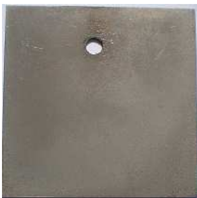
Fig. 3 Appearance of correct nickel-coated tin with opaque coat at electrical energy generation from PV panels
