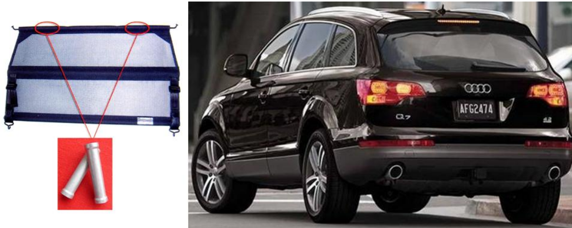
Fig. 6. Aluminum foam crash energy absorber mounted into the dividing net of Audi Q7 developed by IMMM SAS
