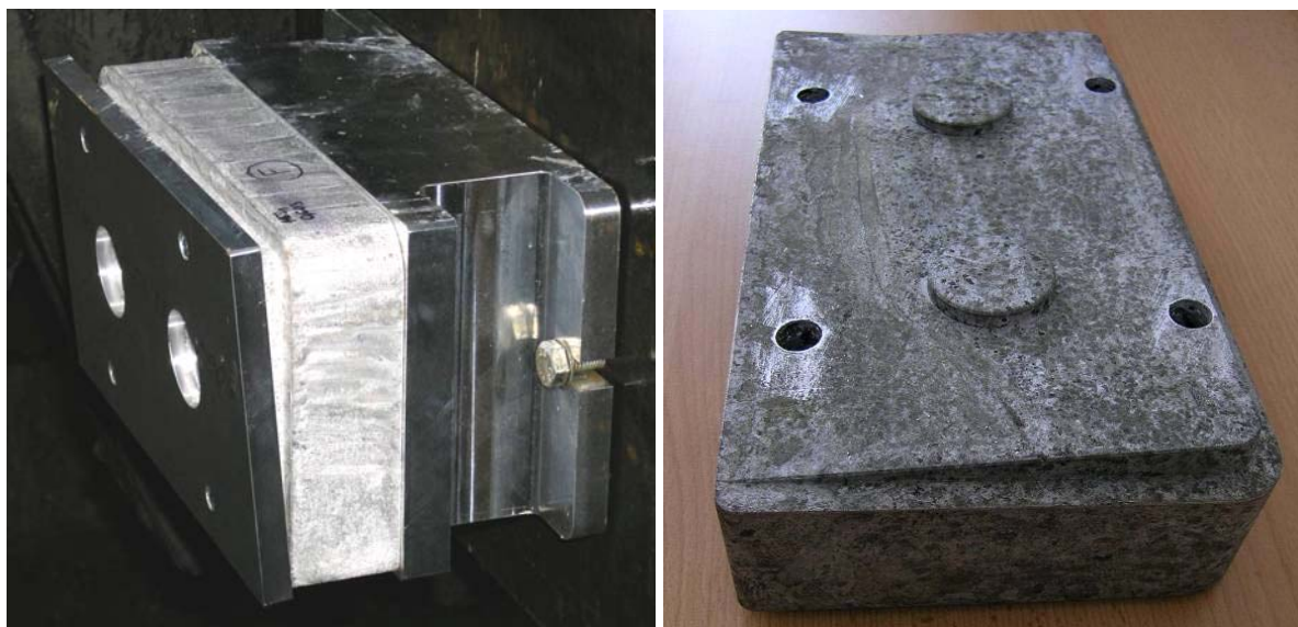
Fig. 5. Assembled crash box containing Al foam (left) and Al foam component (right) Al-foam component for automotive application produced in high volume series
