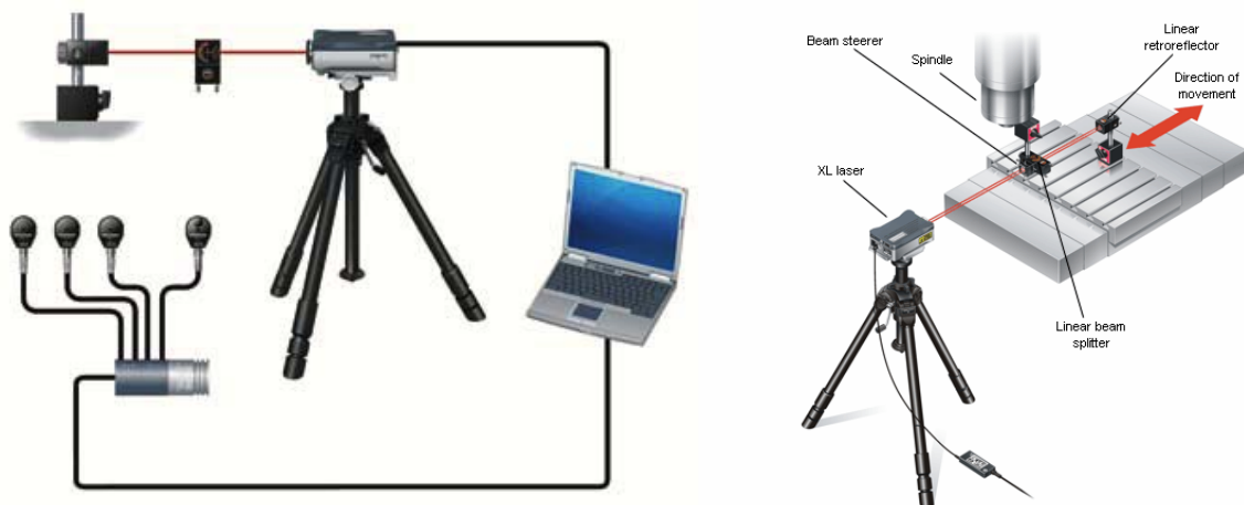
Fig. 2. Renishaw XL-80 measurement system with XC-80 compensator and sensors
