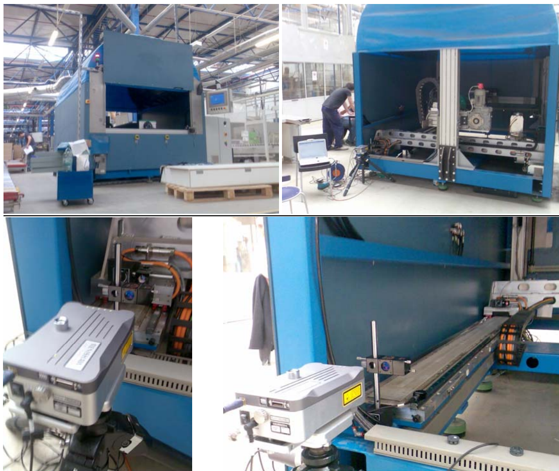
Fig. 7. Linear measuring on control videocheck machine for Ikea factory with using Renishaw XL80
