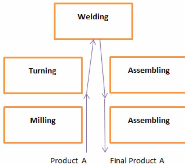
*Fig. 2 One-piece flow manufacturing environment*
