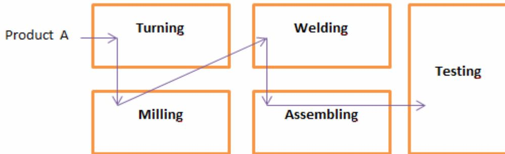
*Fig. 1 Batch-and-queue manufacturing environment*
