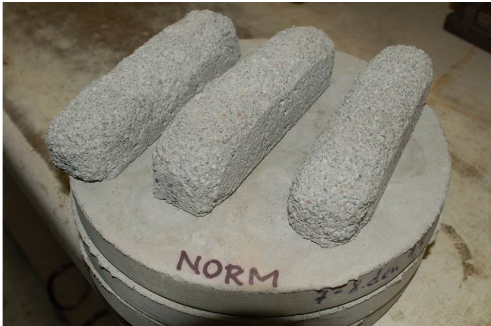
Fig. 3 Cement mortar without hydrofobizer after 50 frost/defrost cycles in presence of salts
