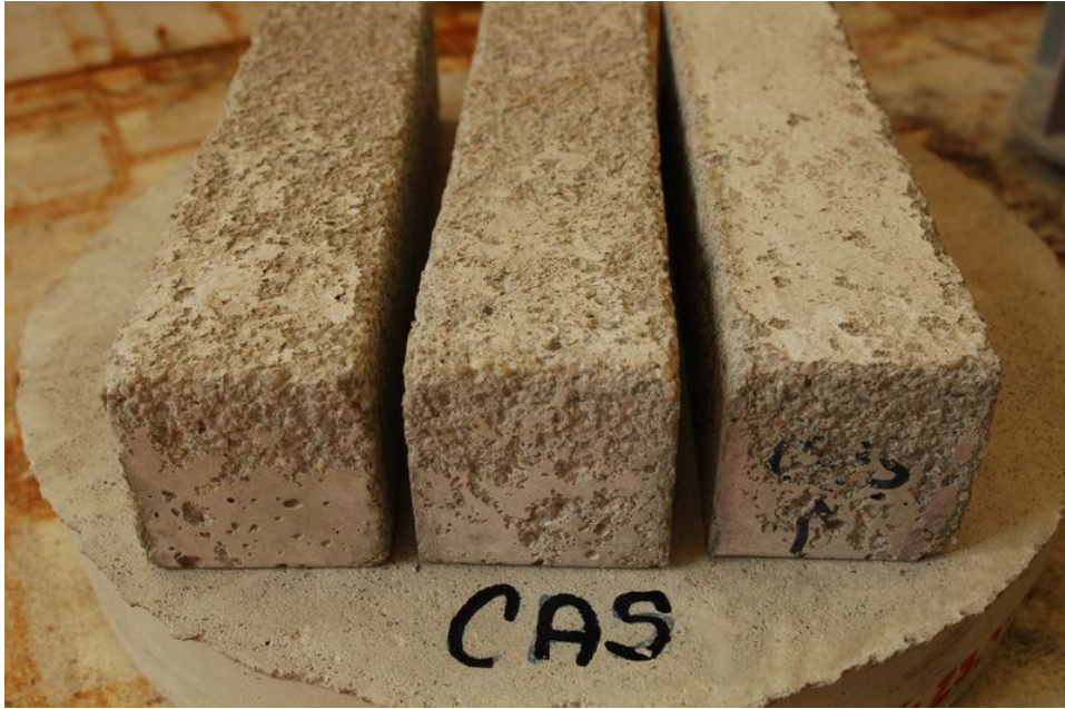
Fig. 2 Cement mortar with Ca Stearate after 50 frost/defrost cycles in presence of salts
