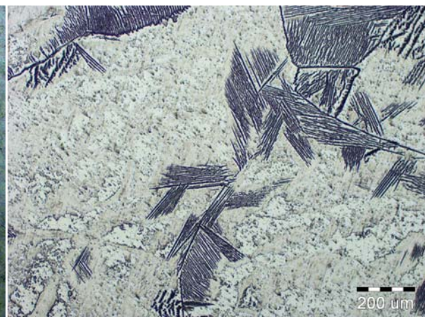
Fig. 7 Lamellar ( \alpha+\beta ) microstructure of Ti-25Nb after annealing
