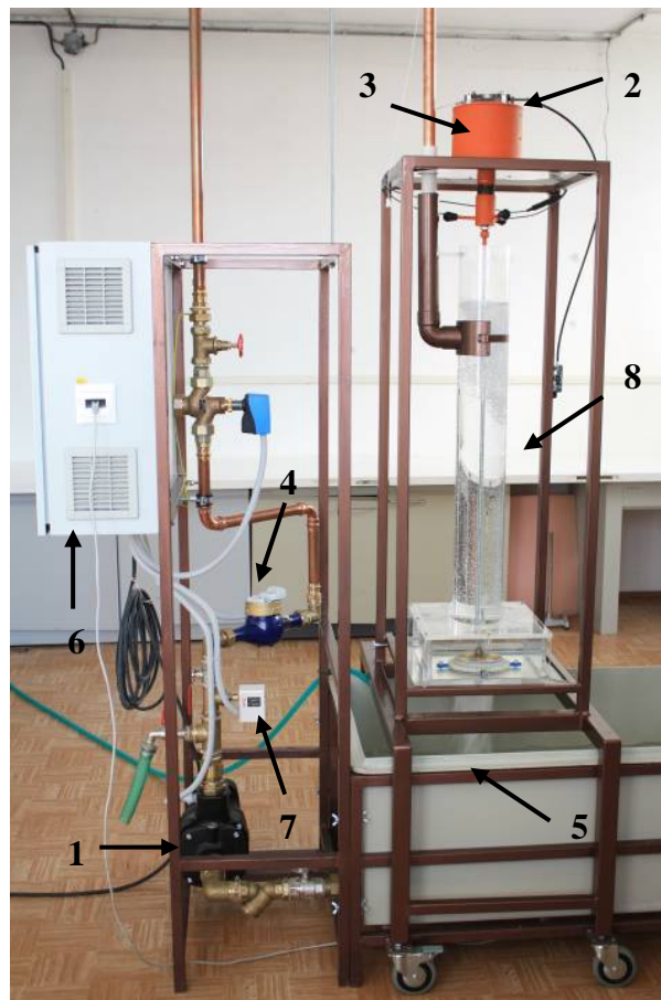
Figure 1 Measuring stand for Pico-hydropower plants [Photo by authors]
