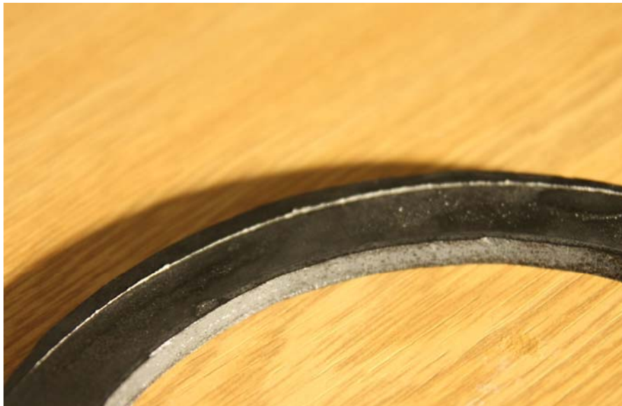
Fig. 2 The cover gasket of electrolyser is without visible damage [Photo: R. Kuracina]
