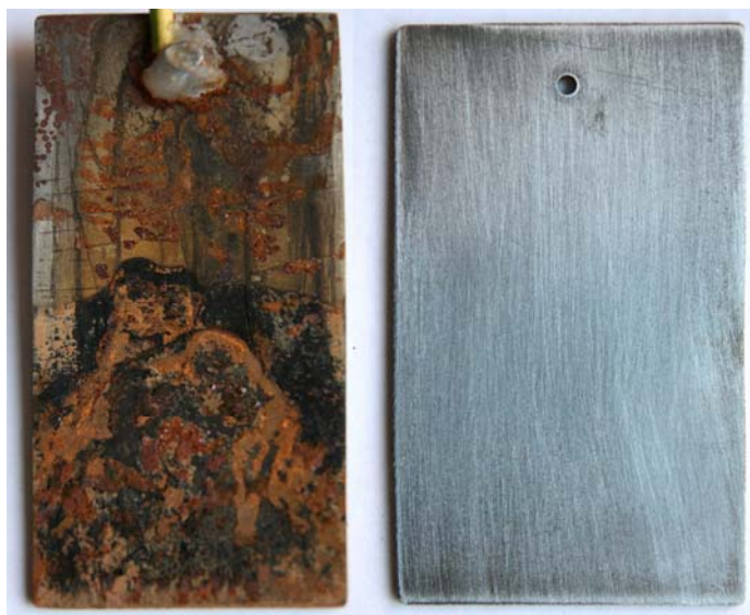
Fig. 4 Damage of iron electrode used as anode [Photo: R. Kuracina]
