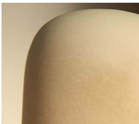
Fig. 7 Detail of the diaphragm surface after 6 months in electrolyser [photo: R. Kuracina]
