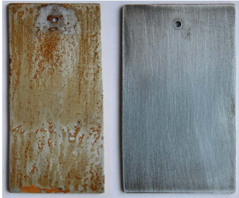
Fig. 3 The result of long-term influence of electrolyte on iron electrode (left) [Photo: R. Kuracina]
