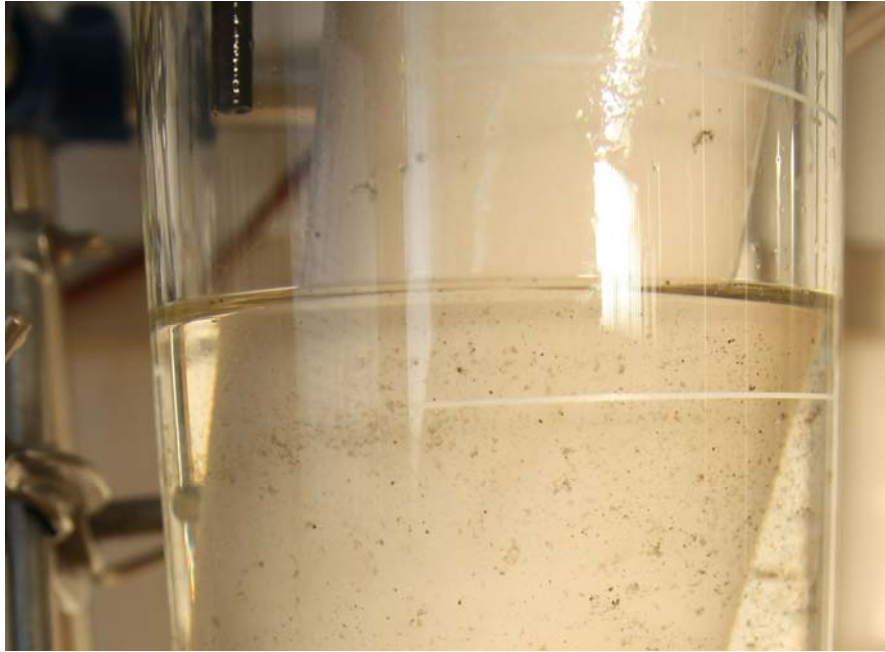
Fig. 1 Glass body of electrolyser evinces no signs of destruction [photo: R. Kuracina]
