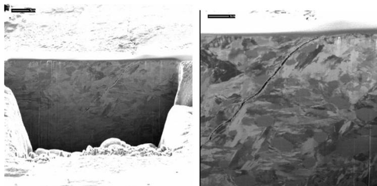
**Fig. 6** FIB/XB-Investigations at the outer end of the elliptic wear mark (width of the complete cut is about 20  $\mu\text{m}$ , the visible depth is about 10  $\mu\text{m}$ )
