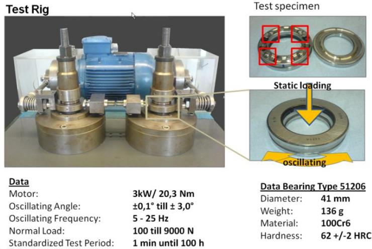
**Fig. 3** Test rig with standard test parameters
