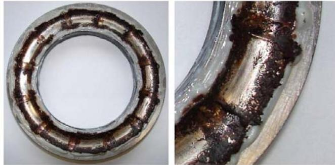
*Fig. 1 Axial ball bearing with advanced damage*
