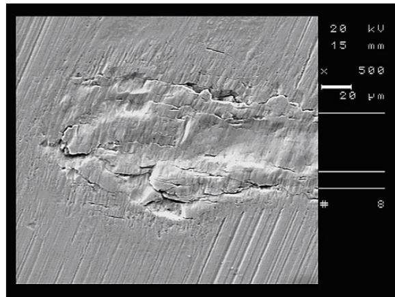
**Fig. 5** SEM picture of the outer end of the elliptic false brinelling mark of a high (!) reference grease after just 1000 load cycles
