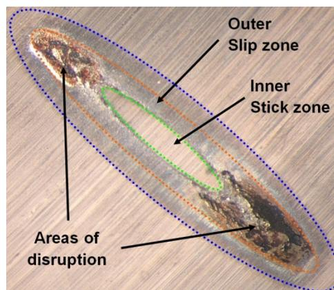
**Fig. 4** Division of the marks in different contact zones like stick zone, partial slip zone with micro sliding and affected zone (from the inside outwards)
