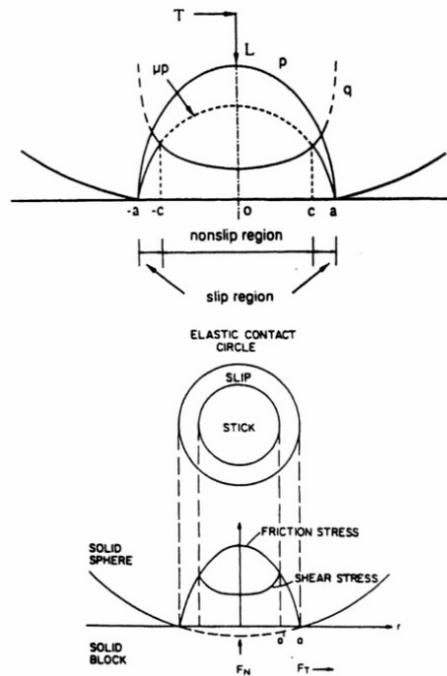
*Fig. 8 Microslip in a point contact with acting tangential force (1)*
