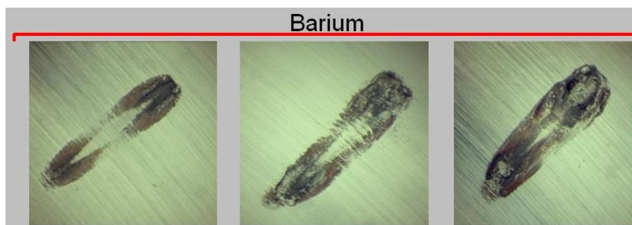
*Fig. 7 Marks after 1 min., 6 min. and 80 min. with a barium soap grease*
