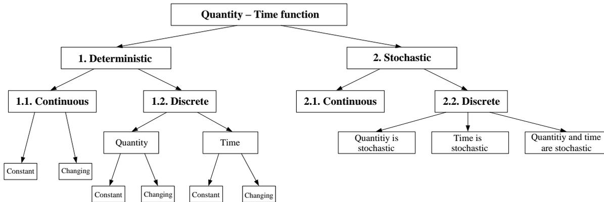
*Fig. 3. Alternative material flow-time functions*
